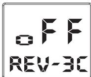
**Setting up the 3<sup>rd</sup> Channel:** Press MENU function Left key (<) (Press once under MAIN MENU), then press twice on Menu function Right key (>) until you see \*\*\*REV-3C, press DATA function Left key (+) or Right key (-) to choose ON/OFF. (Screen shows OFF REV-3C).
