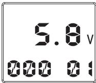
Switch on the transmitter, you will hear “beep” sound (beeps once), and the LCD display mode will read the default parameters pre-set at the factory and BATT status mode (main menu).
