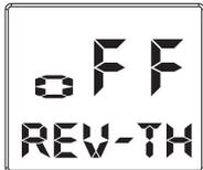
**Setting up Throttle speed neutral position.** Press MENU function Left key (<) (Press once under the MAIN MENU) and then press twice of MENU Right key (>) until you see \*\*\*REV-TH. Press DATA function Left key (+) or Right key (-) ON/OFF. (Screen shows OFF REV-TH).
