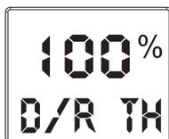
**Set up Throttle servo (TH) forward and reverse angle.** Press MENU function Left key (<) (Press 3 times on MAIN MENU), then press MENU function Right key (>) once, the screen shows \*\*% D/R TH, press DATA function Left key (+) or Right key (-) for throttle angle parameters. (Screen shows 100% D/R TH)
