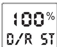
**Set up Steering servo (ST) angle.** Press Menu function Left key (<) (Press 3 times on MAIN MENU) until you see \*\*% D/R ST on the screen, then press DATA function Left key (+) or Right key (-) to choose servo angle parameter. (Screen shows 100% D/R ST).
