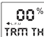
**Setting up throttle speed (TH) neutral position parameters.** Press MENU function Left key (<) (Press twice under MAIN MENU), and press MENU function Right key (<) until you see \*\*% TRM TH and neutral value. At this point, press DATA function Left key (+) or Right key (-) for adjustment. On the screen you will see neutral position status indicator L. F. U, R. B. D and percentage values. (Screen shows 00% TRM TH)
